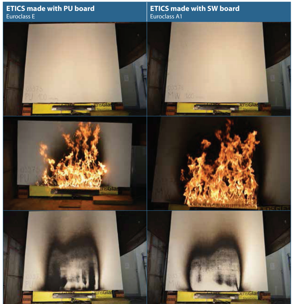
Photos taken before, during and after the tests on two samples of the cladding systems
